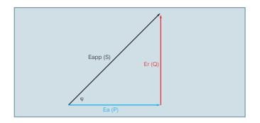
• Active energy (Ea): expressed in kilowatt hours (kWh). This can be used, after being transformed by the receiver, in the form of work or heat. The active power P (kW) corresponds to this energy.
